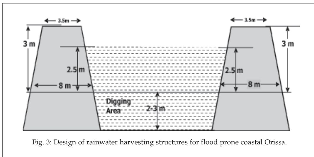
Fig. 3: Design of rainwater harvesting structures for flood prone coastal Orissa.
