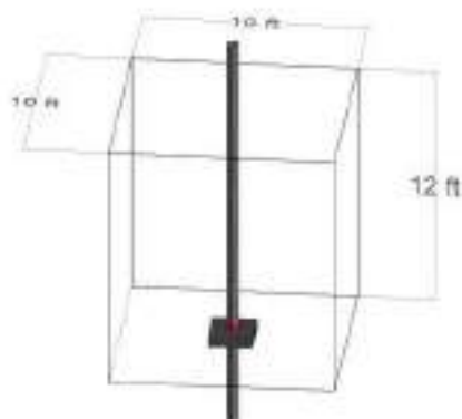
Fig. 2. Cross-sectional view of the secondary filter of the pit filtration technique
