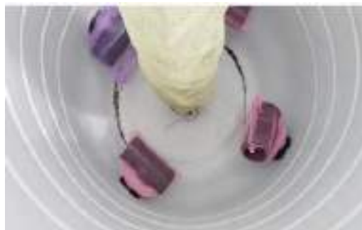
Fig. 3. PVC T-s covered with screen inside plastic tank
