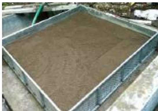
Fig. 2. On-line screen gravel filter functioning with layer of sand filter
