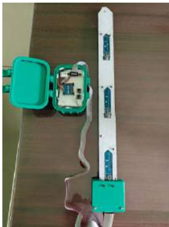
Multi-depth (up to 54 cm) soil moisture sensing unit
