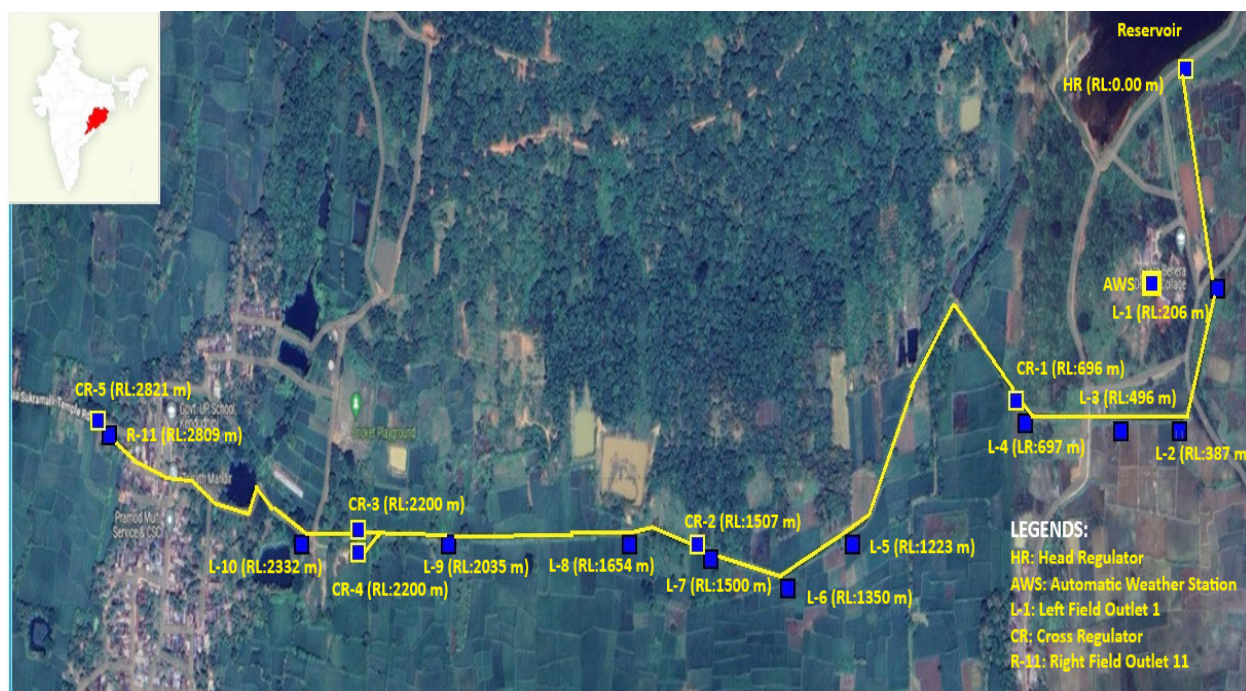
Fig.3 The detailed layout with automated outlets, head regulator and cross regulators in the entire stretch of the MI command.
